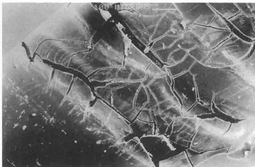
FIG. 18. Crack pattern on inner lumen of polyether urethane lead insulation tracking coil indicative of metal ion-induced oxidation. \times 100 .
