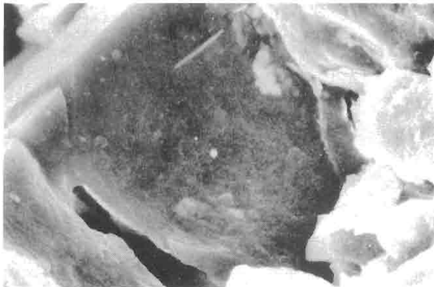
FIG. 17. Smooth crack wall indicative of brittle fracture caused by metal ion-induced oxidation. \times 830 .
